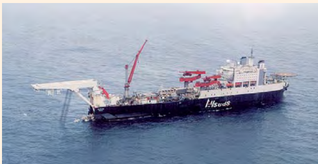
Allseas' dynamically positioned pipelay vessel Solitaire
